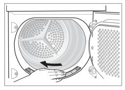
After a period of time, a gleam due to detergent residue on laundry forms on the filters. When this occurs, clean the filters with warm water using a brush. Remove the filter from the door pulling it out. (It can be positioned with the locating spur facing to the left or to the right).
